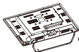
3. screw the base and connected to the TV.
